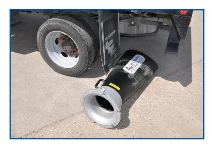
Polymer horns can be manipulated by hand back into shape if accidentally damaged due to crushing or bending.
